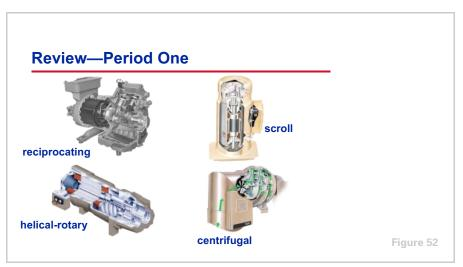
Period One introduced the four types of compressors commonly used in airconditioning applications: reciprocating, scroll, helical-rotary (or screw), and centrifugal.
